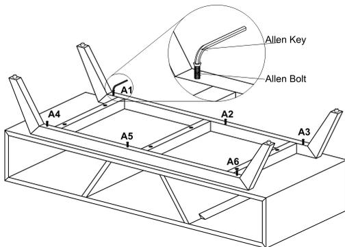
Fix the PART-B(leg) with Allen Bolt using Allen Key at position A1,A2,A3,A4,A5&A6 as shown in Fig.
